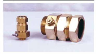
Cable Glands with an integral earth connection are recommended for use with high voltage systems. The earth connection on these glands has been successfully tested in accordance with the 43kA short-circuit test specified in BS 6121, Part 5, 1992.
